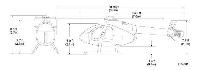
Figure 1-1. MD 520N Principal Dimensions - Standard Landing Gear
